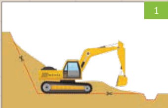
1 Levelling and drainage excavation are done according to the project. Geocell and other materials are installed.
